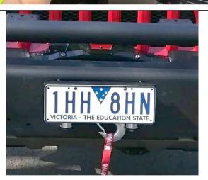
Fit number plate to number plate bracket using 2x M6x16mm hardware provided (if applicable).
