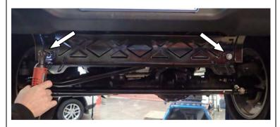
3. Remove 2x M10 SEMS from the steel front panel and discard.
