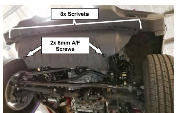
2. Remove 2x 8mm A/F Self Tapping Screws from the plastic Splash Panel below the Bumper.
