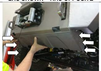
Fit under panel to outside of uprights using 6x M8 button head bolts and flange nuts provided.
