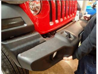
8. Remove OE Bumper and integrated steel impact beam from vehicle and discard.
