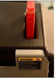
Fit recovery point decals to under panel directly below recovery points as shown.
