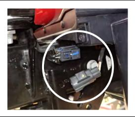
4. Disconnect fog light harness, located on the RHS chassis rail, access from inside wheel arch.
