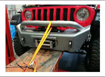
24. With the assistance of a second person and/or height adjustable trolley, carefully position the bar in front of the chassis mounts, taking care to route any winch or other accessory cables around obstacles and clear of the chassis mounting faces.
